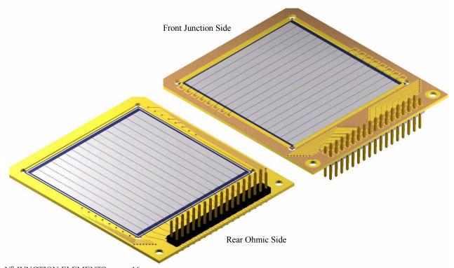
$\begin{array}{lll} N^{\circ} \ \ JUNCTION \ ELEMENTS: & 16 \\ N^{\circ} \ OHMIC \ ELEMENTS: & 16 \\ ELEMENT \ LENGTH: & 49.5 \ mm \\ ELEMENT \ PITCH: & 3.1 \ mm \\ ELEMENT \ WIDTH: & 3000.0 \ \mu m \\ ACTIVE \ AREA: & 50.0 \ x \ 50.0 \ mm^2 \\ CHIP \ DIMENSIONS: & 52.25 \ x \ 52.25 \ mm^2 \\ 53.78 \ x \ 53.78 \ mm^2 \end{array}$
