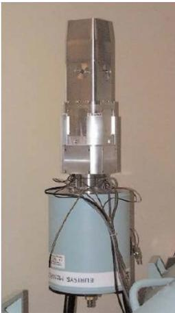
A segmented detector can be used to measure the **linear polarization** which can be used to distinguish between magnetic (M) and electric (E) character of radiation of the same multipolarity.
